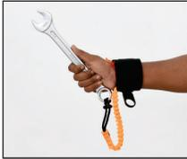
Always make sure the hook-and-loop closures fasten properly, because they make sure the bracelet stays closed and holds if the tool is dropped.
