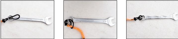
⇒ Always properly tie the knot made using the stopper on the cord.
