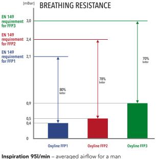
**Inspiration 951/min** – averaged airflow for a man doing harder work while breathing in/inhale. Breathing resistance is measured in millibars – mBar.
