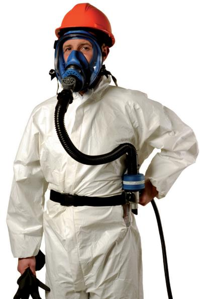
The **TR 2002 CL2** full face mask with panoramic visor is connected to the overflow valve that releases the excess air to the external environment. The mask is fed by the **TUR 60** corrugated hose which drives breathable air in the respiration zone and which is positioned between the overflow valve and the filter silencer connected to the flow regulator.
