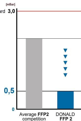
Half-mask that has one of the lowest breathing levels on the market. Air flow of 95l/min is the approximate value of breath when working in heavier environments
