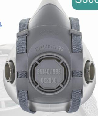
The S600 respirator can be used with filters, absorbers and filter absorbers: 701 A1, 702 A1E1, 703A1B1E1K1, 702 A1E1P3R, 703 A1B1E1K1P3R, 793 P3, 793C P3 with an active carbon layer and with 2000, 5000 and 6000 series.
